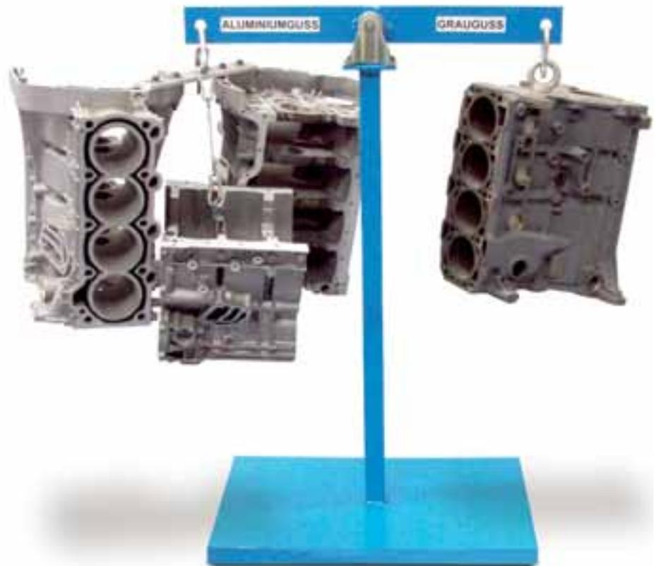
Fig. 1 Double pan balance aluminium vs. grey cast
